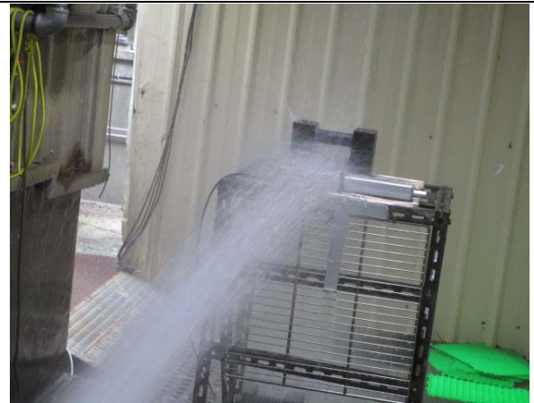
Photo H: Test setup (Waterproof test)
